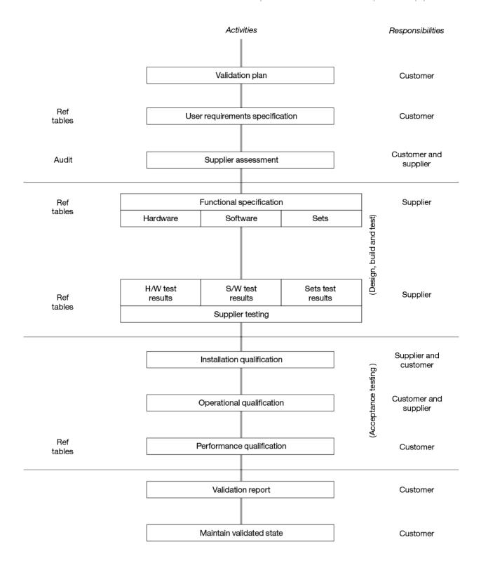
Figure 8.1 Generic flowchart of apheresis equipment acceptance
